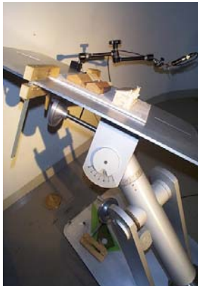
A Heliodon simulates solar exposure and shading
